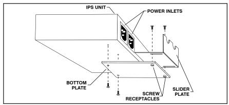
Figure 4.1: IPS-800 Series Cable Keeper Installation
